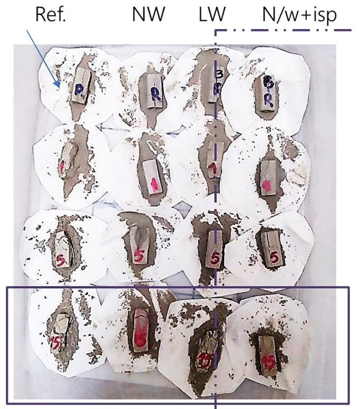
Fig. 9 Degradation patterns of treated and untreated briquettes, subjected to water absorption
