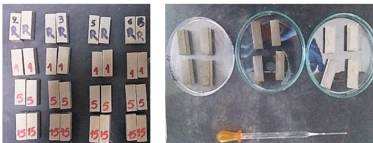
Fig. 3 Laboratory synthesized clay briquettes, with different montmorillonite content and application procedure of the consolidation treatments
