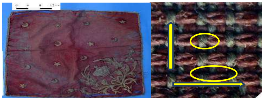
Fig 2. The historic fabric (left); microscopic image of the red crimson ground fabric showed the both the lengthwise and crosswise yarns in different colours(400x).
