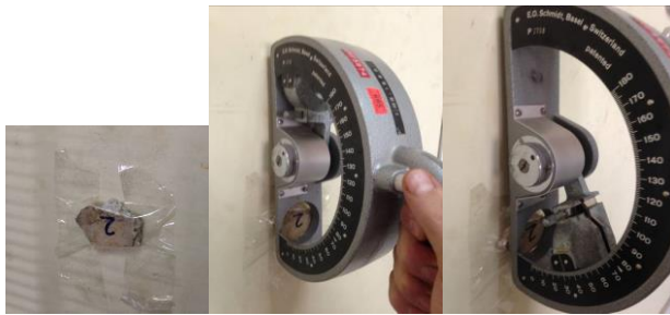
Figure 6. Surface hardness measurement of P2 specimen with Pendulum type Schmidt hammer (Sound specimens with no damage after pendulum hammer hit)
