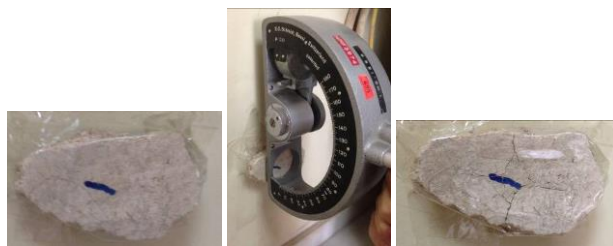
Figure 7. Surface hardness measurement of P1 specimen with Pendulum type Schmidt hammer (Crushing and fracture of specimen after pendulum hammer hit)
