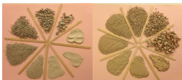
Figure 10. Aggregates of a) BBM and b) BWM mortars sieved by ISO 565 series meshes (8, 4, 2, 1, 0.500, 0.250, 0.125 and 0.063 mm). All aggregates of BBM and BWM passed 8 mm meshes.
