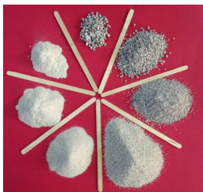
Figure 9. Aggregates of P1 plaster sieved by ISO 565 series meshes (4, 2, 1, 0.500, 0.250, 0.125 and 0.063 mm). All aggregates of P1 passed 4 mm meshes.
