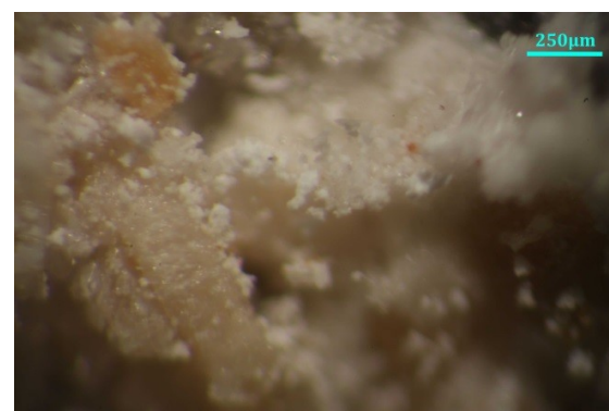
Figure 3. Optical microscopy pictures of mortar FR3M; a whitish mortar with a high content of lime binder and much fluorescence on its surface.
