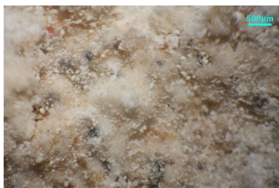
Figure 3. Optical microscopy pictures of mortar FR3M; a whitish mortar with a high content of lime binder and much fluorescence on its surface.
