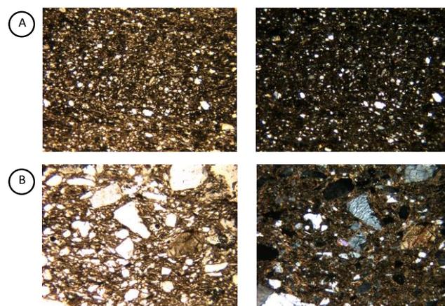
Figure 3. Thin-sections of the ceramic samples (x 230). A: Sample with fine texture (HD-8). Light: white light- Right with cross light. B: Sample with coarse texture (HD-6). Light: white light- Right with cross light
