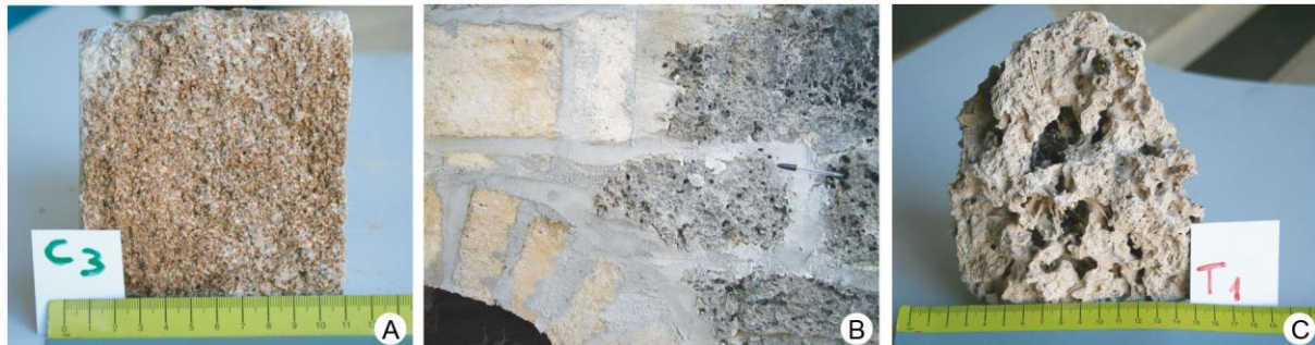
Figure 4. Illustrations of the carbonate material used before (c) and after (a) the restoration. (b) difference between the two materials after the restoration (calcarenite on the left; calcareous tufa on the right).
