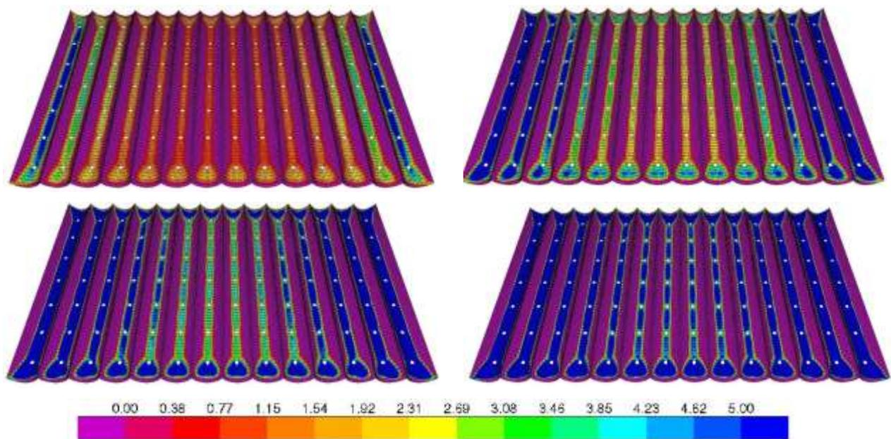
Figure 28. The effect of increasing filling depth on the maximum principle stresses in the vaults’ inner face in the magazines of Ramesseum temple. The cases from top left to bottom right are: self-weight (OW), OW+1m of filling, OW+2m of filling and OW+3m of filling, respectively.
