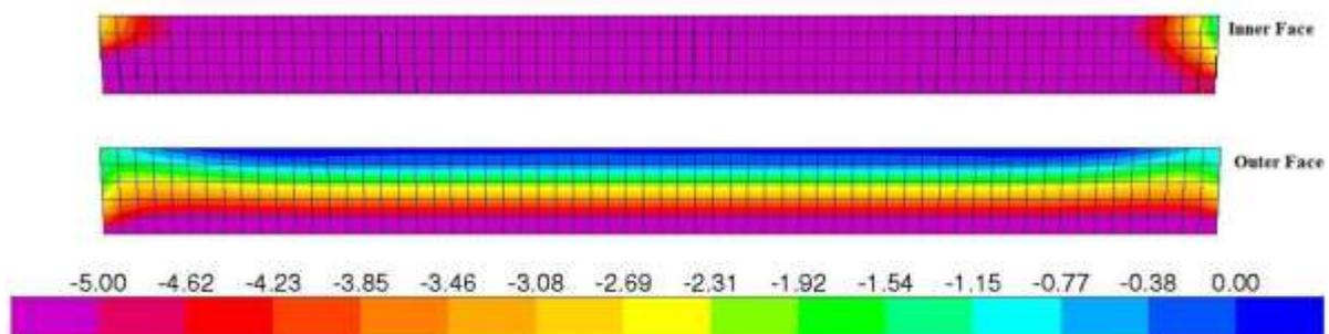
Figure 24. Locations of the minimum principle stresses (compressive stresses) (t/m<sup>2</sup>) in the walls of the typical bay of the Ramesseum magazines: at the inner face of the wall (top) and in the outer face of the wall (bottom).
