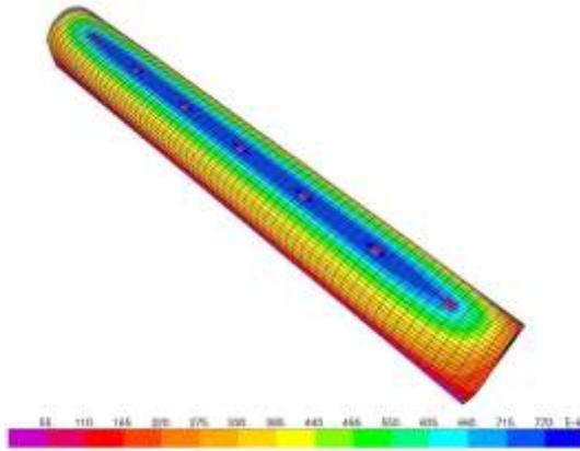
Figure 21. Resultant deformations (m) of the typical bay of the Ramesseum magazines.
