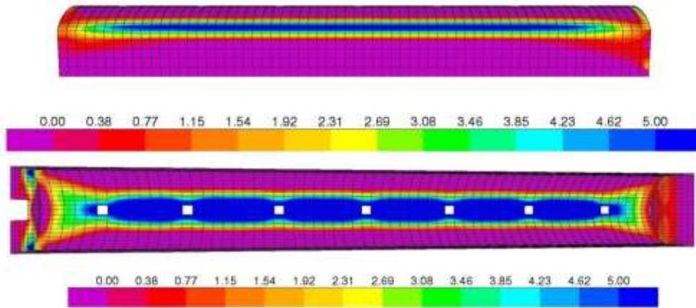
Figure 22. Locations of the maximum principle stresses (tensile stresses) (t/m<sup>2</sup>): at the outer face of the vault springing (top) and the bottom face of the vault mid span (bottom).
