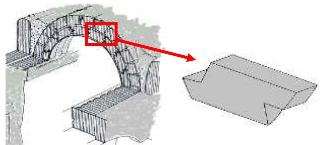
Figure 6. Adobe vault in Ancient Egypt composed by two courses. The bricks were specially designed with interlocking edges, used over the chapel in the tomb of Sabef (6th Dynasty) at Giza (after Fisher, 1924).
