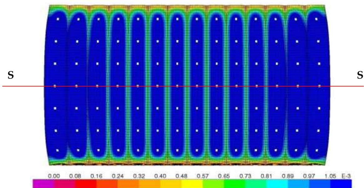
Figure 26. Resultant deformations (m) of the magazines of Ramesseum temple, case of self-weight+1 m of filling. The red line indicates the place of the transversal section in the vaults "S-S".
