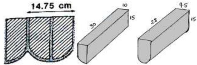
Figure 4. Bricks with curved sides made specifically for vaults construction. Discovered in a chapel of 4<sup>th</sup> dynasty in old Kingdom in Giza (after Fisher, 1924 and Spencer, 1979a).
