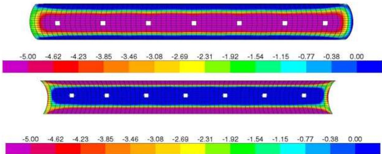
Figure 23. Locations of the minimum principle stresses (compressive stresses) (t/m<sup>2</sup>) in the vault of the typical bay of the Ramesseum magazines: at the outer face of the vault mid-span (top) and the inner face of the vault springing (bottom).
