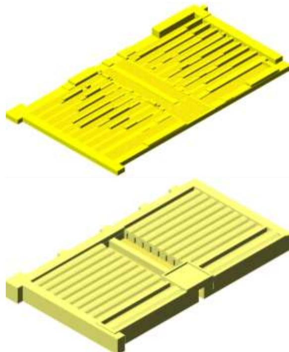
Figure 33. The documentation of the current state of collapse of the Sety I storerooms (top) and a 3D view of the proposed reconstruction (bottom) (after, El-Derby, 2005, figs. 224, 281).
