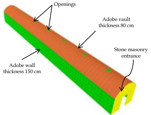
**Figure 20. 3D model of the typical bay of the Ramesseum storerooms. Different colors indicating different thicknesses or different materials.**
