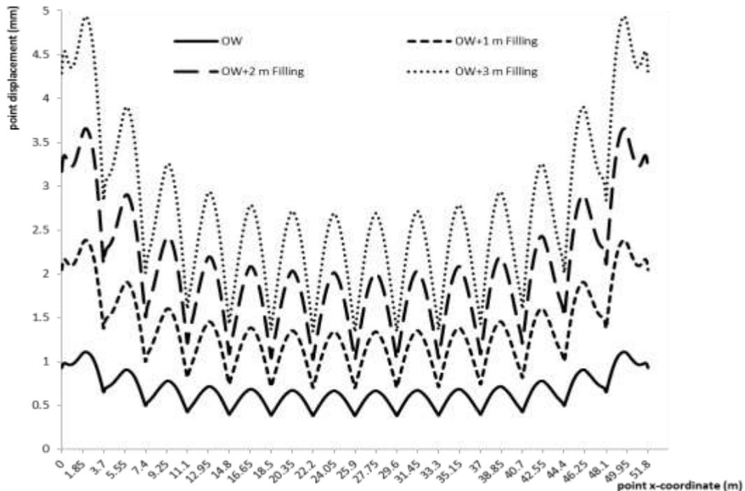
Figure 27. The effect of increasing filling depth on the Resultant deformations (m) of a selected transversal section “S-S” in the magazines of Ramesseum temple. OW=self-weight.
