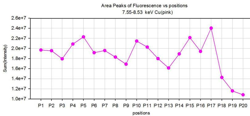
Figure 6. Fluorescence peaks of copper in the 20 points analysed on dagger TS.14.143.
