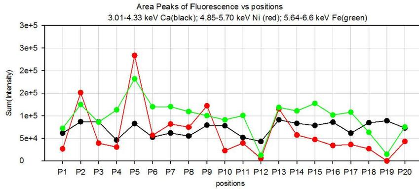
Figure 5. Fluorescence peaks of metals in the 20 points analysed on dagger TS.14.143.
