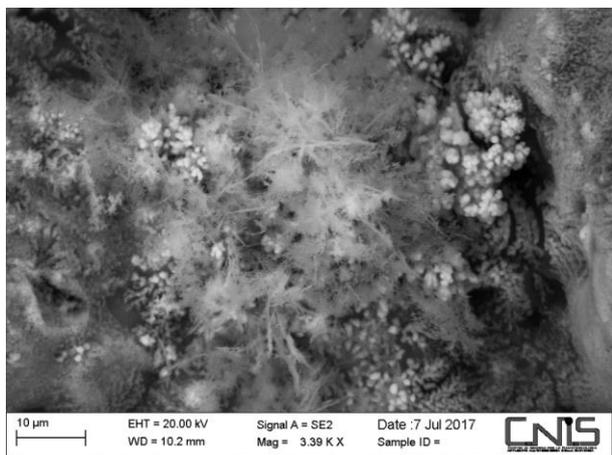
**Figure 9. Magnification at SEM of area where Sn was detected on dagger TS.14.143.**
