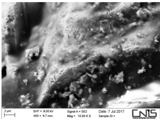
**Figure 10. Magnification at SEM of spherical and rod-shaped nanostructures on dagger TS.14.143.**
