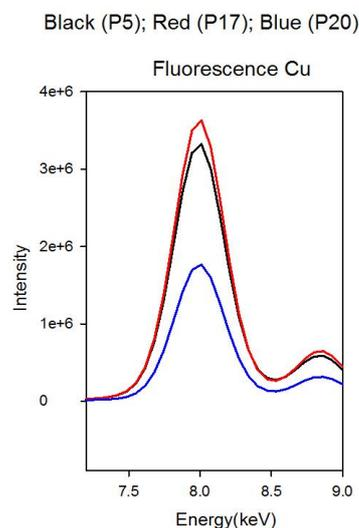
Figure 4. Spectrum of copper on points P5, P17 and P20 sampled on dagger TS.14.143.
