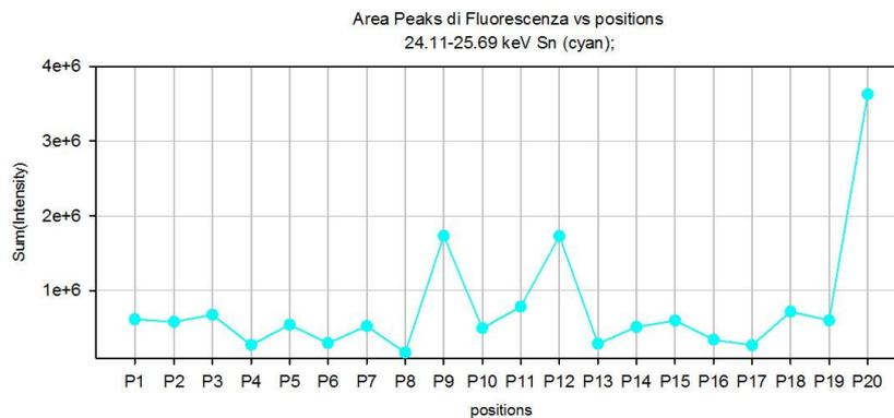
Figure 7. Fluorescence peaks of tin in the 20 points analysed on dagger TS.14.143.
