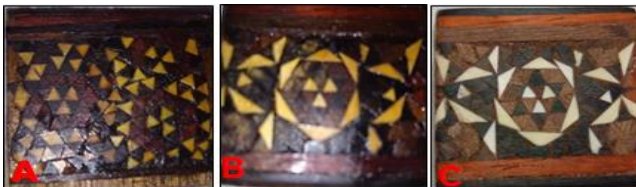
Figure 2 (A)& (B) Manufactured wooden samples after inlay and coating by shellac varnish, (C) Reference sample without coating.
