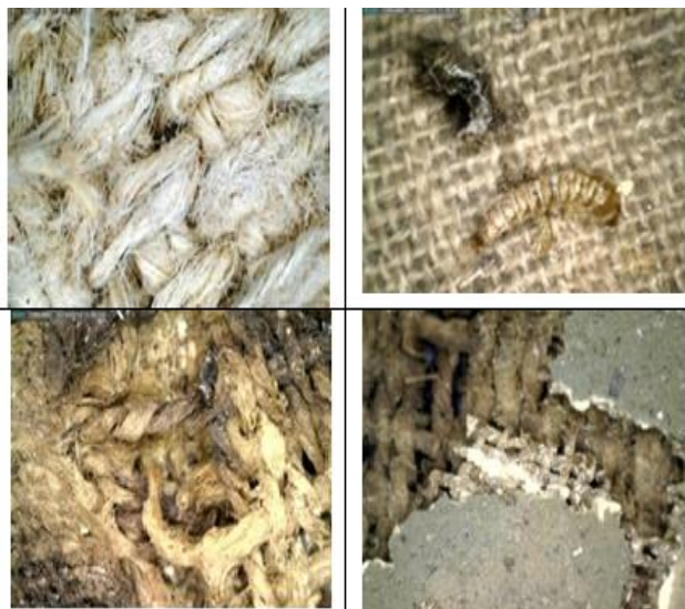
Figure 3. The morphology of fibres under USB microscope, proved that the fibres from linen and the mainly deterioration by insect.
