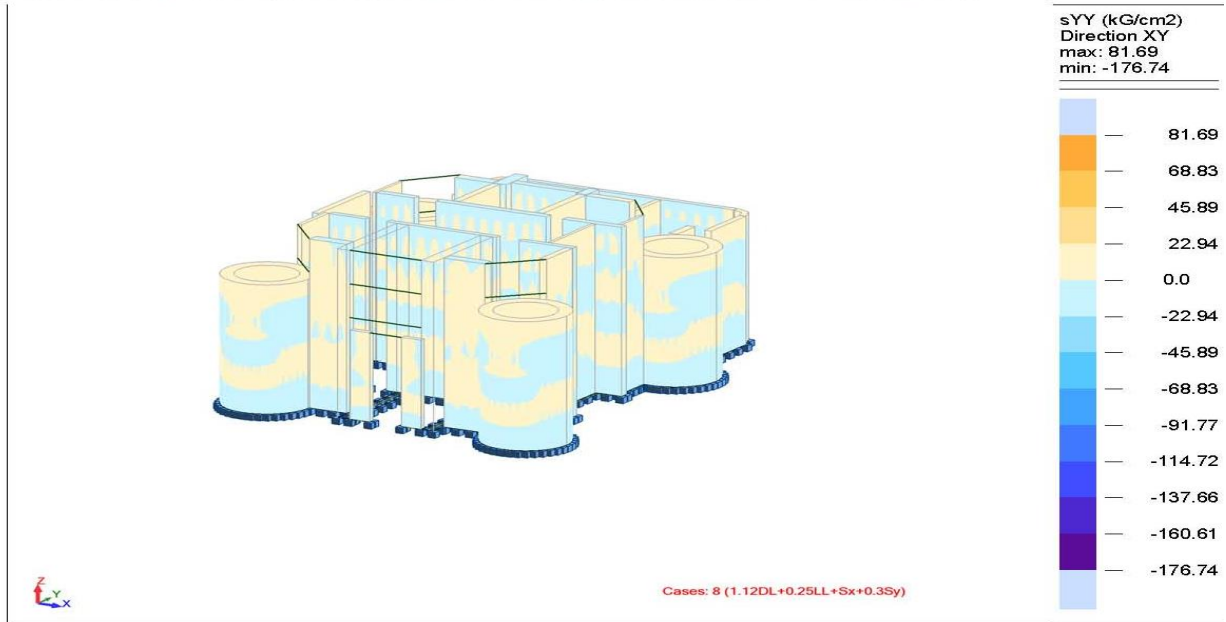
Figure.15. Maps of solids- Effective horizontal compressive stresses \sigma_{yy} (Kg/ cm2) Direction XY cases: (1.12DL+0.25LL+Sx+0.3Sy).
