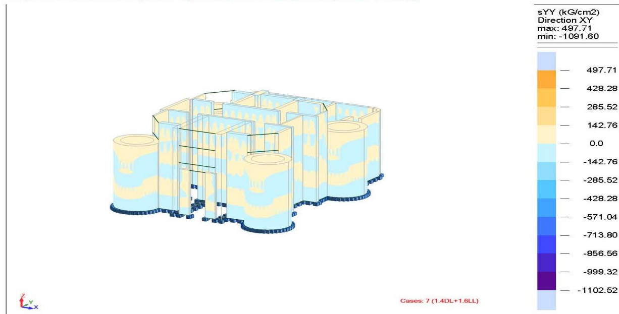
Figure.12. Maps of solids- Effective horizontal compressive stresses \sigma_{yy} (Kg/ cm2) Direction XY cases: (1.4DL+1.6LL).
