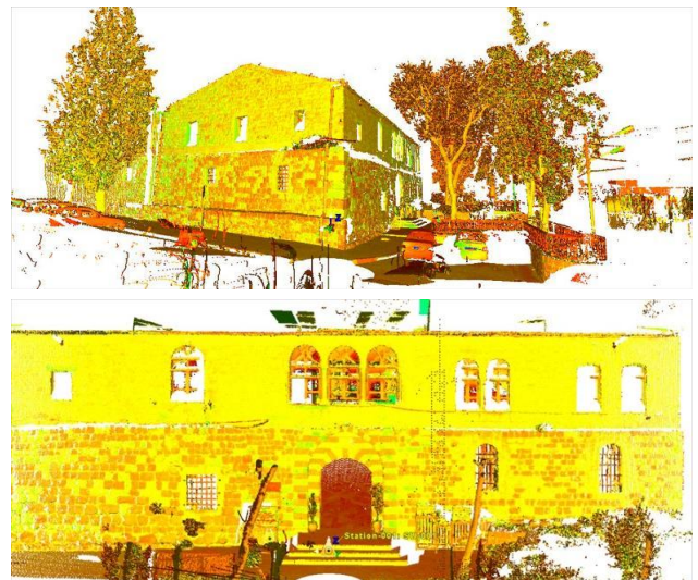
Figure 8: Missed laser point clouds due to obstacles, material type or limited range of view.
