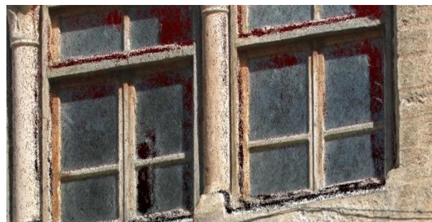
Figure 10: 3D point clouds of the front façade using DSM.
