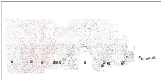
Figure 9: Reconstruct the images positions and orientation parameters using Structure for motion algorithm. The algorithm also generates a sparse point cloud of the faced.
