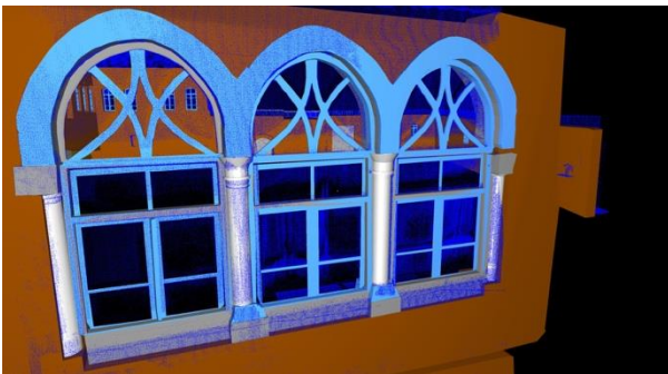
Figure 14: 3D CAD modeling using registered point clouds, the windows were modeled in more realistic and accurate shape.
