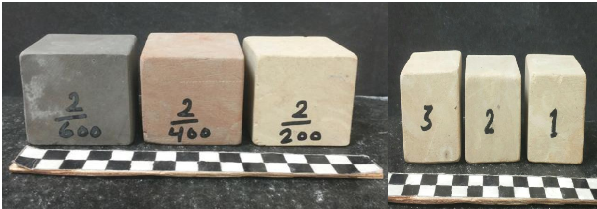
Figure.11. photos showing the colour change of stone samples before and after the fire.
