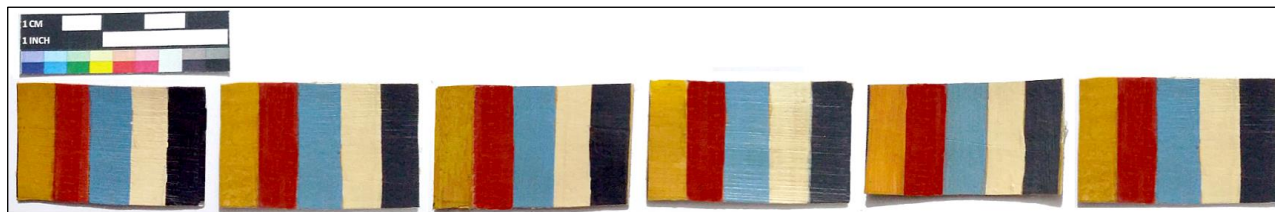
Figure 1. Some prepared SPMs after thermal accelerated aging.
