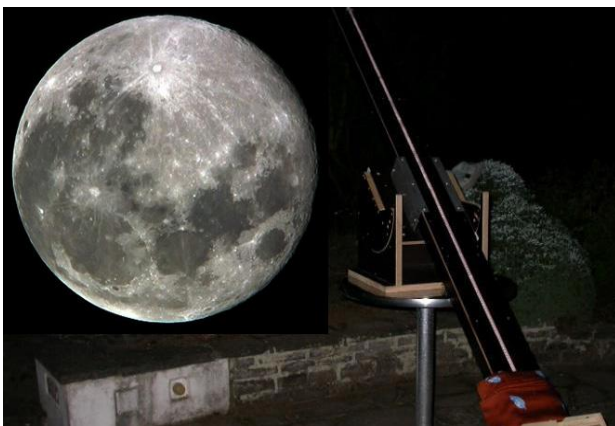
Figure 2: The Herschelian telescope with the obsidian mirror, ready for observing; Full Moon observed with the obsidian mirror. Still image taken from a film. Photos: Josef Vit.
