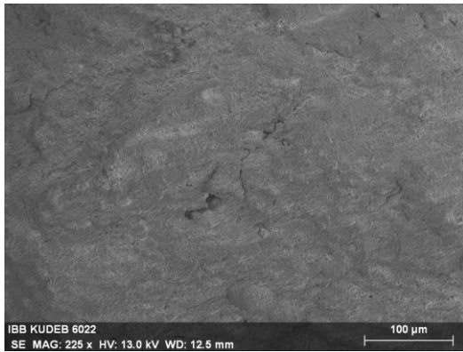
Figure 43. SEM images of micro cracks.
