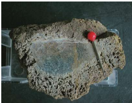
Figure 8. From the Stötttham impact layer: sawed surface of a silica limestone exposed to strong heating. Only a core has retained its original texture. In the outer zone the carbonate has disappeared by decarbonisation and/or melting.
