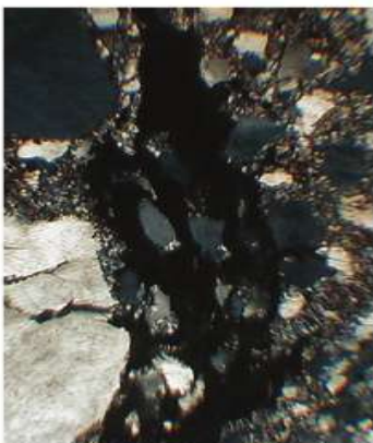
Figure 9. Stötttham diamictite: photomicrograph of a sandstone sample containing glass from probable shock melt – black under crossed polarisers of the microscope. Field width 1.6 mm.
