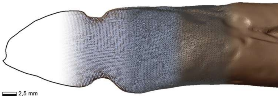
Figure 3 Detail of the 3D digital model of the archaeological artefact D05-KE90-7. To capture the point cloud, we used a non-contact close-range 3D structured light scanner (SmartSCAN3D Duo System, Breukmann), with a 150 mm FOV set of lenses (x,y resolution: 90 µm, according to the manufacturer). From left to right: 2D contour line (shape); 3D point cloud, 3D triangular mesh, 3D mesh with surface, 3D faceted surface (form).
