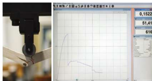
Figure 6 Universal Testing Machine (< 50 kN), using the UNE 56-537-79 standard: Salix sp yield strength test perpendicular to wood grain (left), graphic showing results of yield strength test (right) (Moitinho de Almeida and Barceló 2012a).
