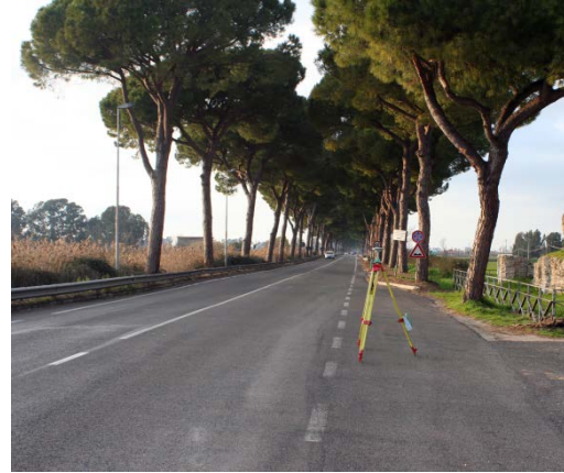
Figure 3. Via Appia at Clesippo's mausoleum in Mesa and the dual frequency GPS receiver (as discussed in the text, the setup did not work properly under dense trees, so the image is only explicative of the working scenario).
