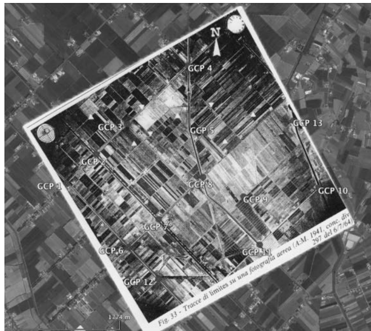
Figure 4. One of the georectified images overlaid on Google Earth, representing an aerial photo (after Cancellieri, 1990) with centuriation traces indicated by triangles; the 13 GCPs used for the georectification (third order polynomials) are also shown; a section of Via Appia extends from the upper left to the lower edges of the figure (crossing GCPs 2 and 7).
