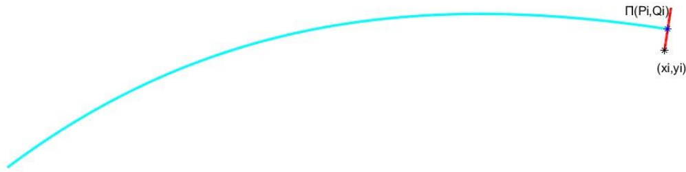
Figure 12. Computation of the distance of the arbitrary point (x_i, y_i) \in CP from GP^{RT} : from this point, we draw the line vertical to curve GP^{RT} , with point \Pi(P, Q) being their intersection. Then, the associated distance is d_{i,GP^{RT}} = \sqrt{(x_i - P)^2 + (y_i - Q)^2} .
