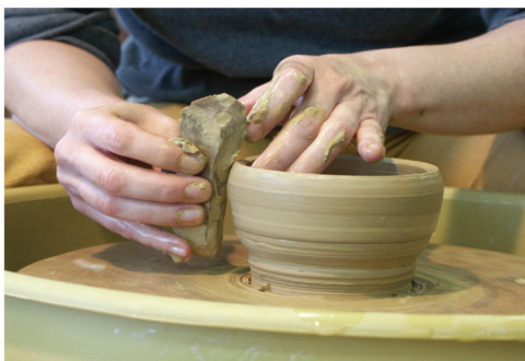
Figure 8. Smoothing and thinning of the wall of a pot made of coarse-tempered clay on a potter's wheel at reduced speed.
