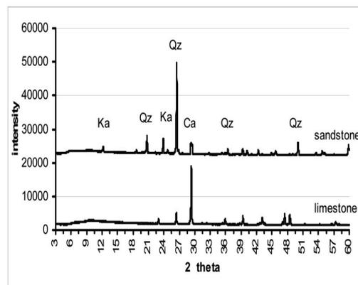
Figure 1: representative powder XRD pattern for sandstone and limestone. Qz is quartz, Ca is calcite and Ka is Kaolinite.
