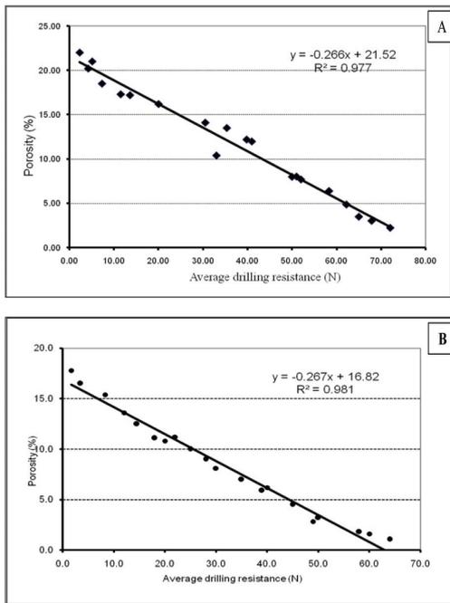
**Figure 2: Scatter diagram showing the reverse linear relationship between porosity (%) and average DR (N) for sandstone (a) and limestone (b).**
