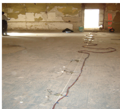
Figure 3. Photograph of the bentonite electrodes and the interconnecting multi cable during data acquisition for tomography A1. Part of the transect in the main praying room is shown.
