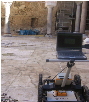
Figure 7. Cart-based Mala system with a 250 MHz GPR in the atrium of the mosque. The instrument is on the ancient floor which was revealed after the excavation. The presence of this floor causes the clear reflection seen in all GPR transects of the first data acquisition phase.
