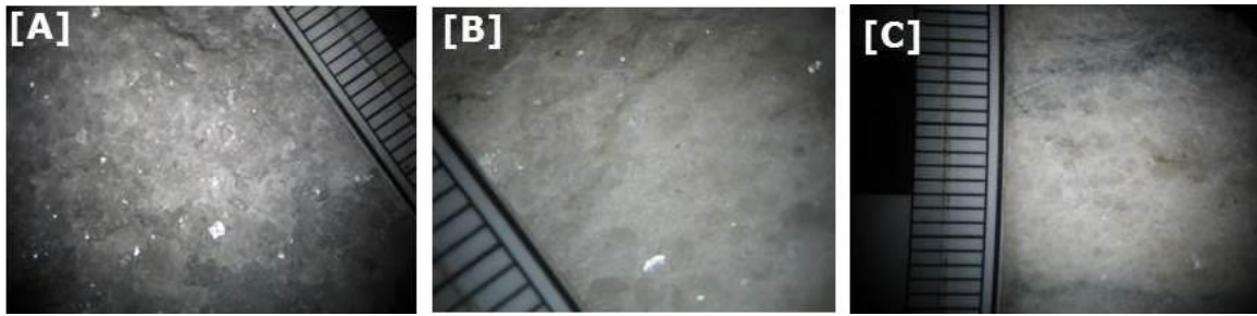
Figure 4: [A] Fine to medium-grained, medium hard marble, [B] Medium-grained and hard marble, [C] Shows dark bands of staining iron-oxides. Scale unit is 1mm.
