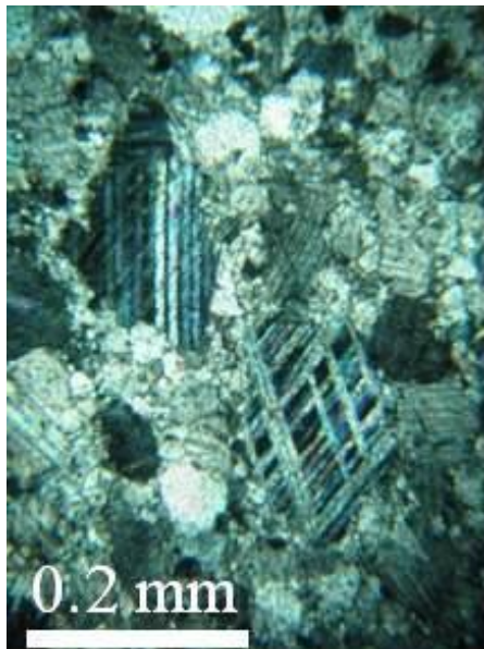
Figure 5: Rhombohedral cleavage in Calcite crystals. 4x, XPL.
